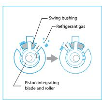
Most manufacturers use a standard rotary compressor, but Daikin, being at the very forefront of energy efficiency and innovation, has improved the technology by developing a swing inverter compressor. This change makes a huge difference in how quiet and efficient the system operates.
