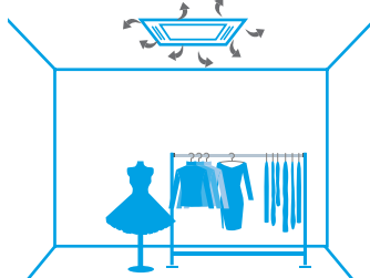
Air distribution with a dusty filter
